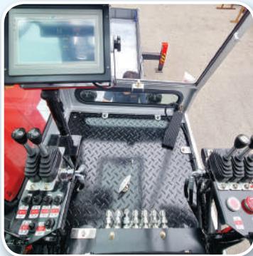
Crane Control Unit at Cabin
